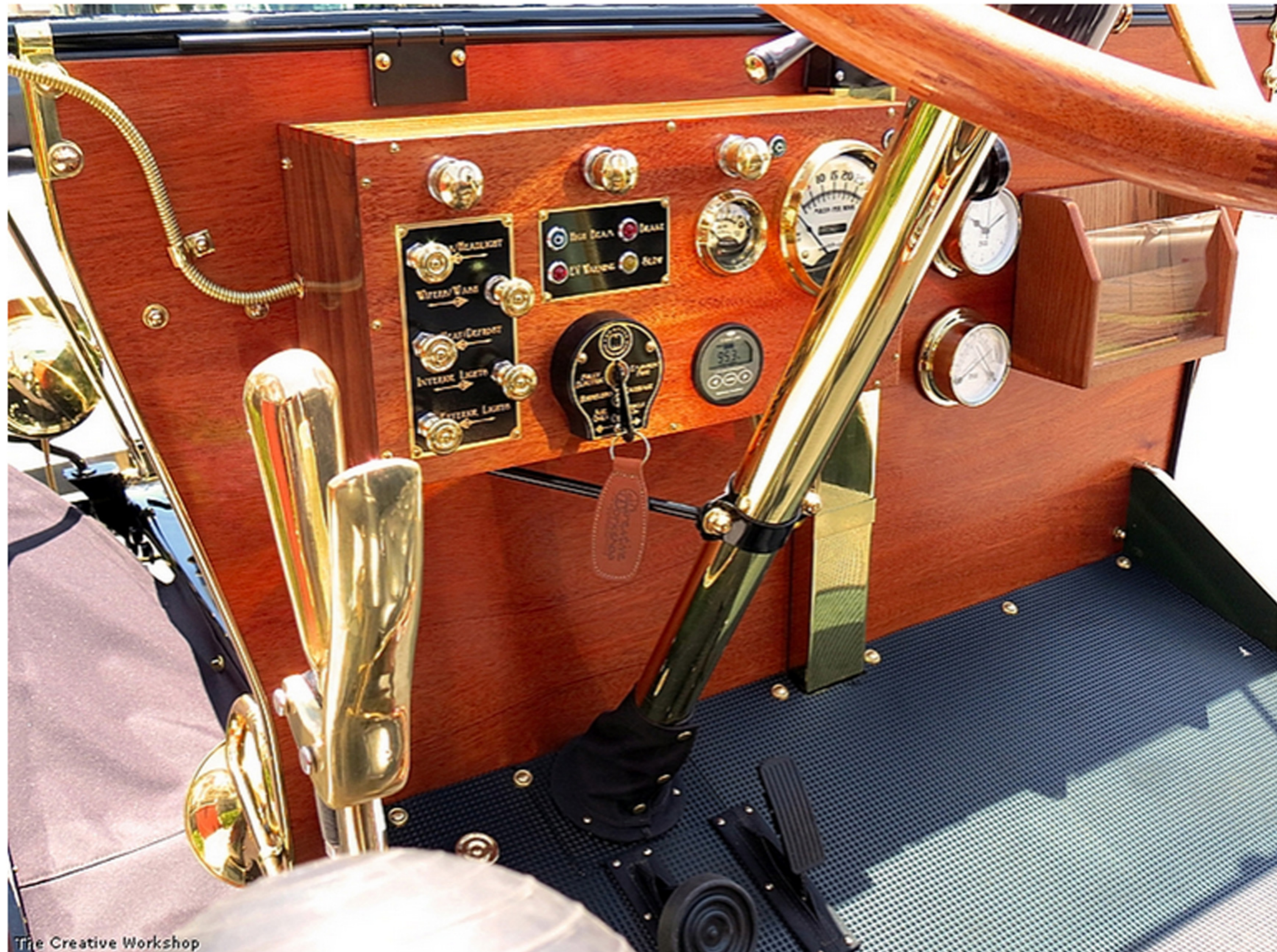
The custom brass hand brake to the left was patterned after one on a WWII military transporter. (Photo credit: The Creative Workshop)
